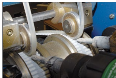
Timing belts with V-guides
