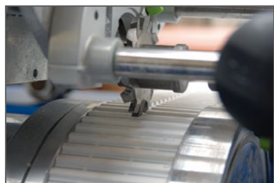
Mechanically processed toothed sides
